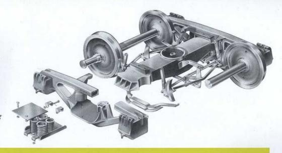
Exploded view of bogie showing arcuate guides with springs withdrawn for examination.
